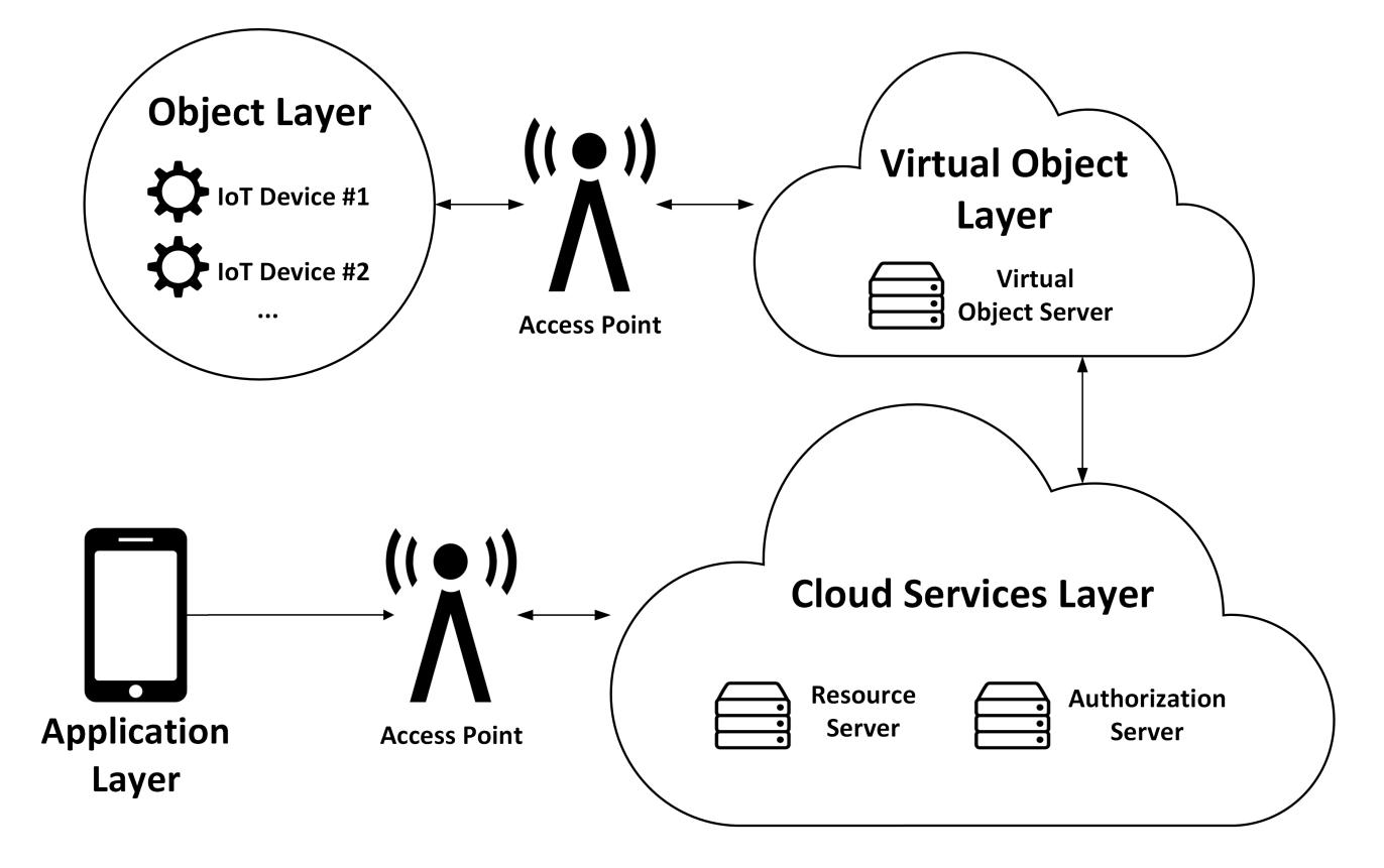
**Application Layer** – Contains applications in the system that can interact with IoT devices and data stored from IoT devices.
